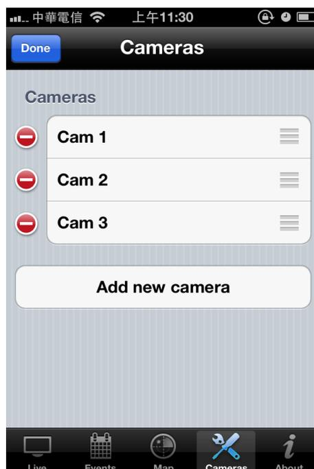
3. If no camera is found, an empty list is shown. Tap “Add New Camera” to manually add a new network camera.
