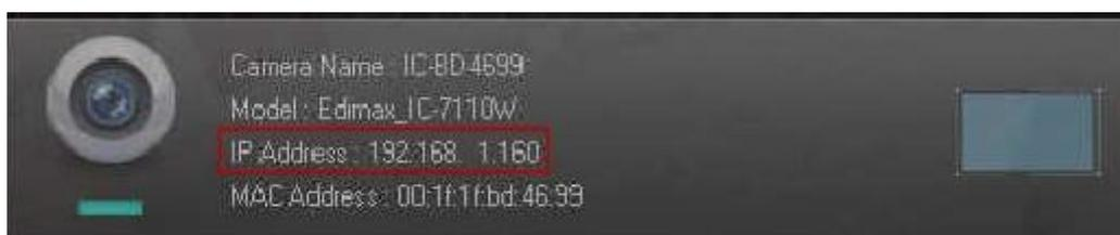
Connection information for a network camera is displayed in each listing under “IP Address”.
